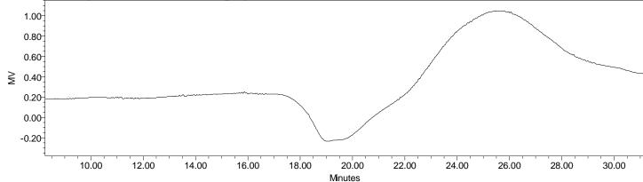
Analysis Method: Waters Breeze system with 1 ml/min DCM flow across three Phenogel 5µm columns (Agilent).
